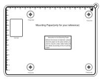
1)Post the mounting template on the wall. Drill holes according to the marks on the template.(Holes for screw and wiring)
