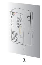
6) Fix the device with the plate after all wiring completed
