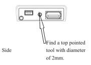
If wrong operation or other unexpected fault makes device fail in working normally, use this function to restart the device.
