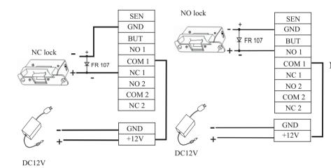
Notice:If lock's working power is DC12V, and working current is least 1000mA less than that of access control device power supply, wiring with sharing power supply can be adopted.
