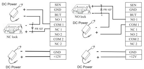
Notice: Wiring with lock power supplied independently is recommended for the following states:
