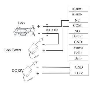
**4.** The output relay signal by Access control station, NO lock connection (Access Control station and lock powered by independent adapter
