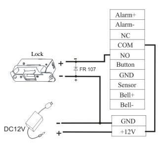
3. The output relay signal by Access control station, NC lock connection (Access Control Station and lock powered by independent adapters jump 1,2 closed)
