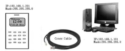
2) Access Control Station connects with PC through network and HUB to create a local network
