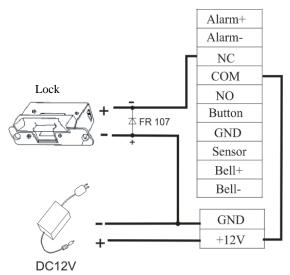
2. NO lock connection (Access control Station and lock powered by one adapter together , Jump 2.3 pin closed).
