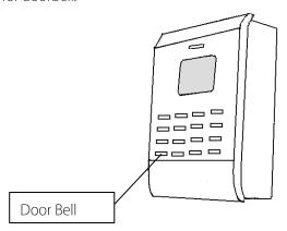
Put the doorbell in the proper place, press the doorbell key on the device, please see circle marked, after the doorbell receive a signal, it will ring.
